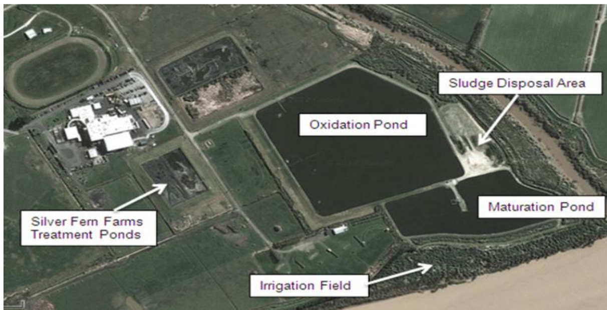
Figure 8-2: Dargaville WWTP layout (KDC Asset Management Plan 2015)
