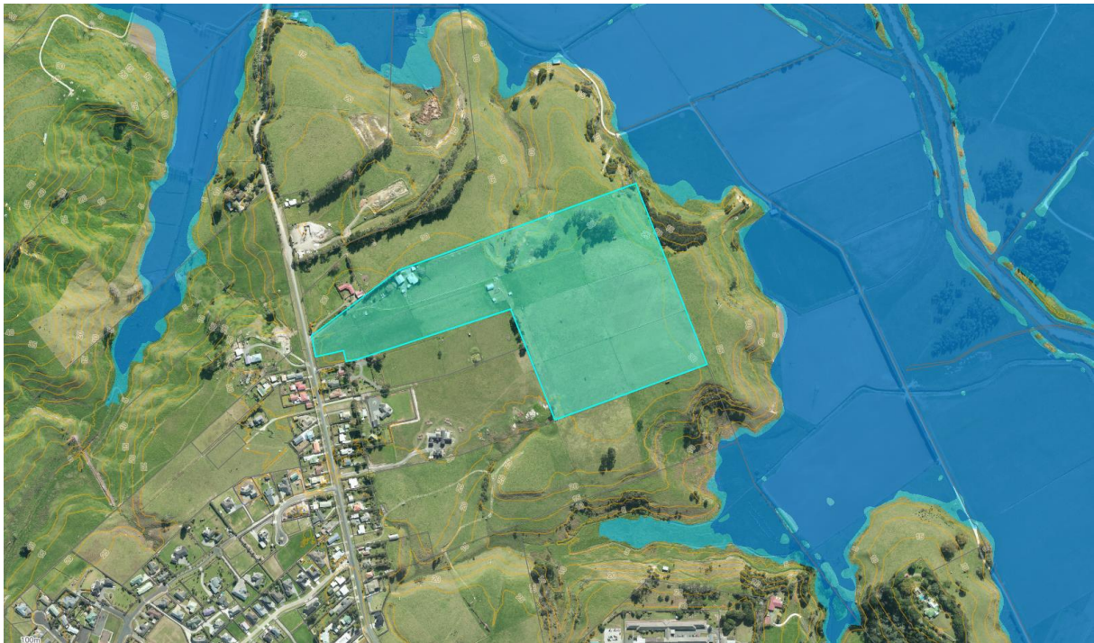
Figure 4-2 Snip of the NRC natural hazards priority rivers flood model – Close Up (accessed 03/03/2022)
